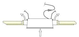
Pull up the spring and put the light into the preinstalled trim.
