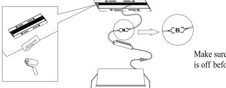
Make sure the power is off before wiring!
